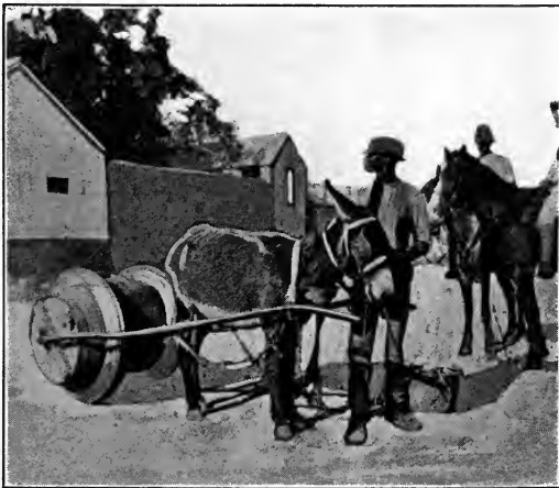
An improvised water-cart, made from a whiskey-barrel, used at Bloemfontein during the water-famine after General De Wet had captured the city's water-works, about twenty miles distant.
